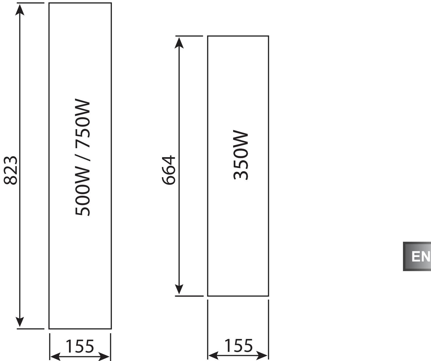
Fig. 1 – Installation aperture
