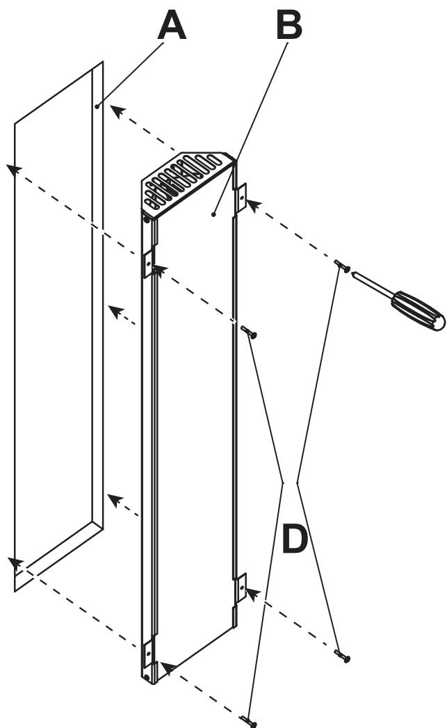
Fig. 4- Installation without screen
